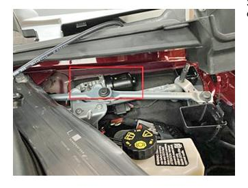
3. Raise the windshield panel cover on the driver's side and record the wiper motor code.
