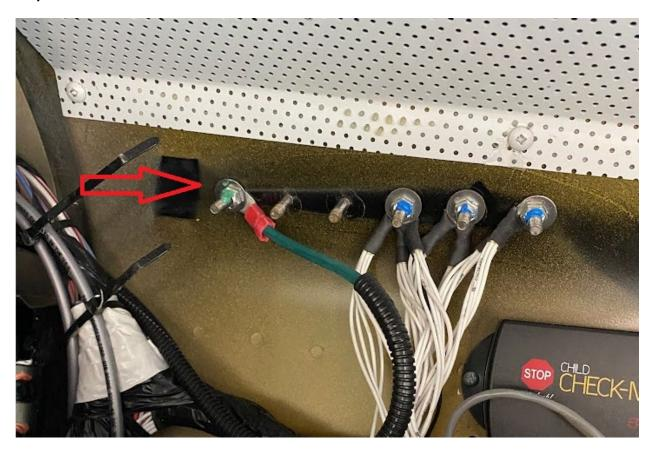
**Ground studs – front side evaporator:** Remove 2 square head screws that hold in place the glove box inner liner located left of driver side overhead compartment. Check nut on the grounding stud for tightness. If loose, tighten (recommended torque 95 in-lbs). If the ground stud happens to break, move the ground to a separate stud. If the nut was not tight, inspect the wiring for any damage – if there is damage to the ground wire, contact TBB for further guidance.
