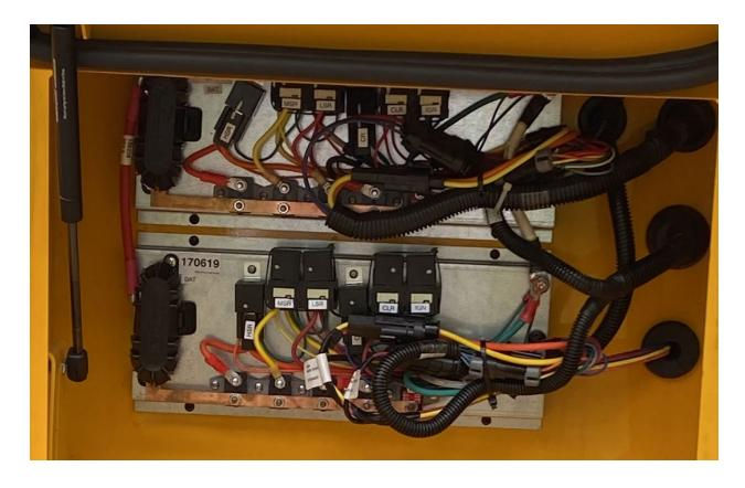
**Connections inside A/C box**: Open the cover of the first door behind the battery compartment. Check for tightness of nuts attaching cables to the BCC control modules. Recommended torque is 95 in-lbs on the B (+) connectors between the cables and the megafuses. Check all connections to the bus bar on the control modules – joints should not be loose – torque nuts connecting wires to bus bar to 24-32 in-lbs if loose. Check all crimped connection joints – wires should be firmly connected.
