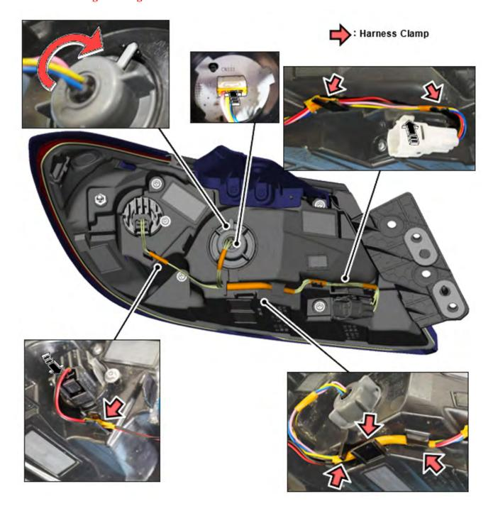
**STEP 10:** Inspect the clip and grommet attached to the body of the vehicle. Confirm there is no loose fitment or physical damage of any kind. If damage is found to the clip or grommet, replacement will be required.
