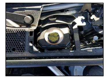
• Inspect brake fluid reservoir cap and replace if necessary.
