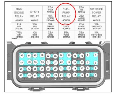
3. With the motorcycle powered off, install the fuel pump relay. Install the fuse box cover.
