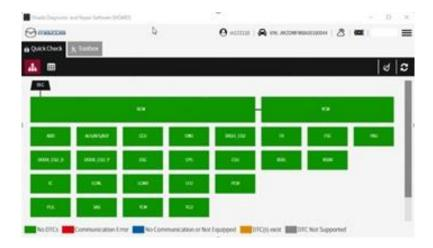
5. Reprogram the "AVAS ISB Amplifier" device as below. At the "Software update" screen on the "Toolbox" tab, select "Run".
