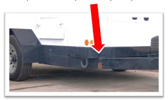
IMPORTANT: For EBB-60 Trailers manufactured between 2020 and 2022, NONE ARE TO BE USED until the trailer has been retrofit with the new EBB trailer tongue assembly. A redesigned and strengthened tongue assembly (65327.400) is being manufactured and will be available this summer.
