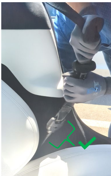
Figure 5 (Pre-tensioner installed correctly, successful pull test)
