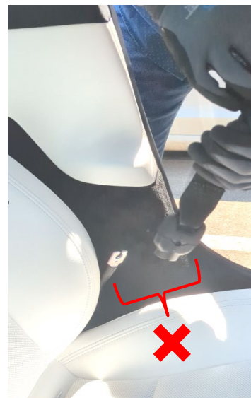
Figure 6 (Pre-tensioner installed incorrectly, unsuccessful pull test)
