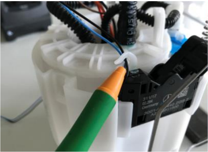
Figure 4 (remove lines from routing clip)
