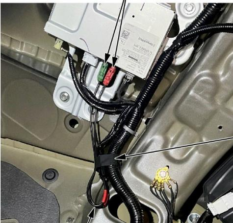
Attach the FAKRA service cables and splice boxes to the appropriate component harness with tape to prevent any rattles.
