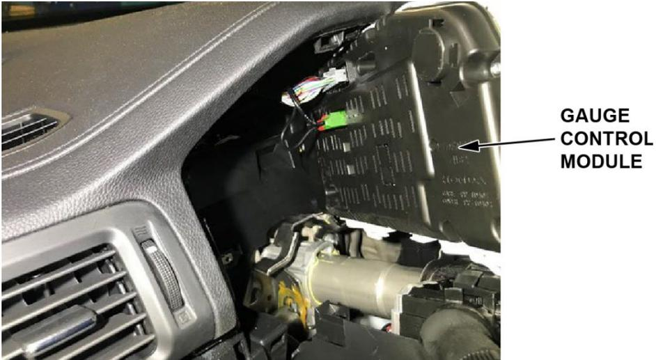
2. Disconnect the red and green FAKRA connectors and any other related connectors from the gauge control module.
