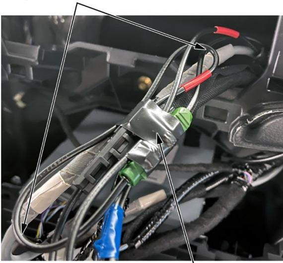
Attach Fakra service cables and splice boxes to the appropriate component harness with tape to prevent any rattles.
