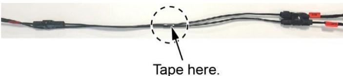
30. Tape the green cable to the single splice box attaching the (green/red) accessory attachment cable to the green FAKRA splice repair cable.
