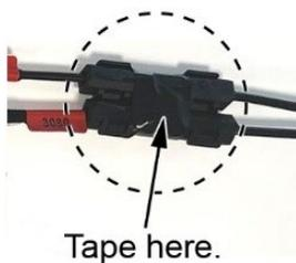
29. Tape the accessory attachment cables together at the midpoint between the two attached 90° splice boxes and the single splice box attached on the green cable.
