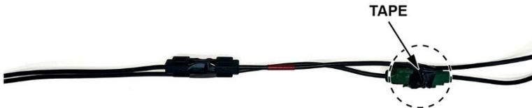
9. Connect the green FAKRA splice repair service cable and splice box to the vehicle dash harness green connector cable.
