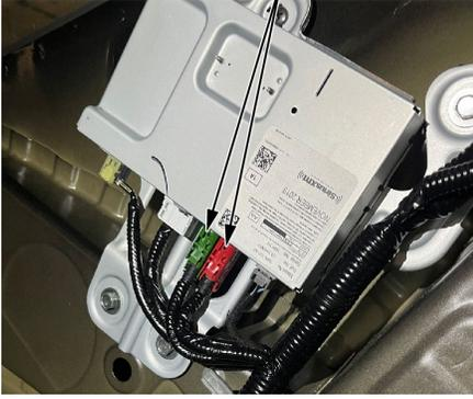
2. Install the matching color FAKRA splice repair service cables and splice box.
