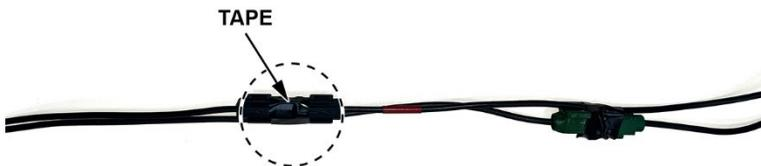
8. Tape the red 90° accessory attachment cable to the green connector.
