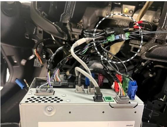
Tape both splice boxes, green connector and cables to the infotainment control unit.
