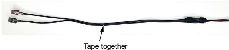
7. Tape the green 90° accessory attachment cable to the splice box.
