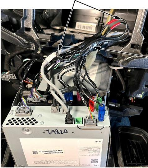
Attach FAKRA service cables and splice boxes to the appropriate component harness with tape to prevent any rattles.
