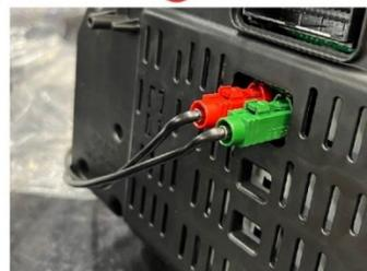
8. Once you have confirmed the cable routing is correct, install the Infotainment Control Unit mounting screws.
