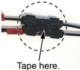
29. Tape the accessory attachment cables together at the midpoint between the two attached 90° splice boxes and the single splice box attached on the green cable.
