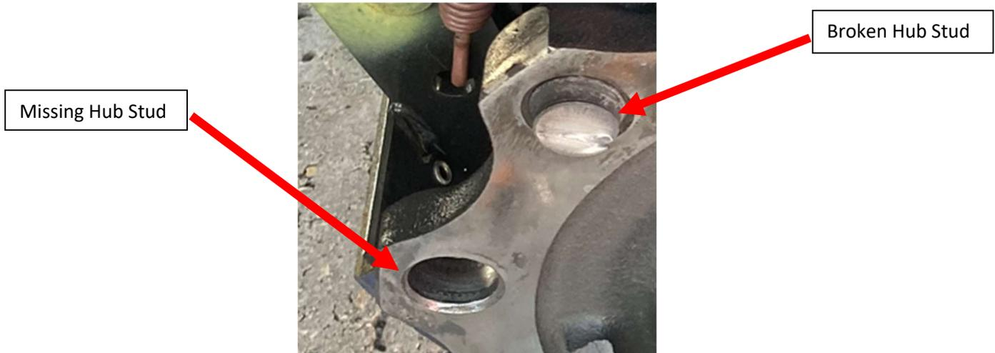
If the stud appears bent or deformed on either side of the hub, this can lead to damage of the stud seats, as seen below, which will lead to loosening of lug nuts and eventually hub failure. Therefore, the stud must be removed.
