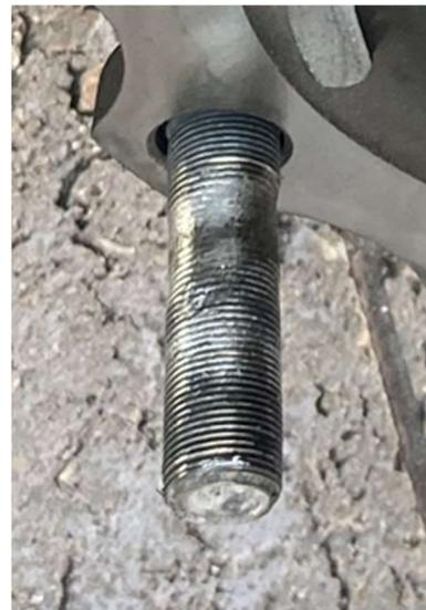
Upon inspection, if any stud appears to have been bent, unseated, necked, stripped, broken or is missing from the hub, it must be removed, and further inspection of the hub must follow. An example of damaged, corroded, stripped and necked studs is shown below.
