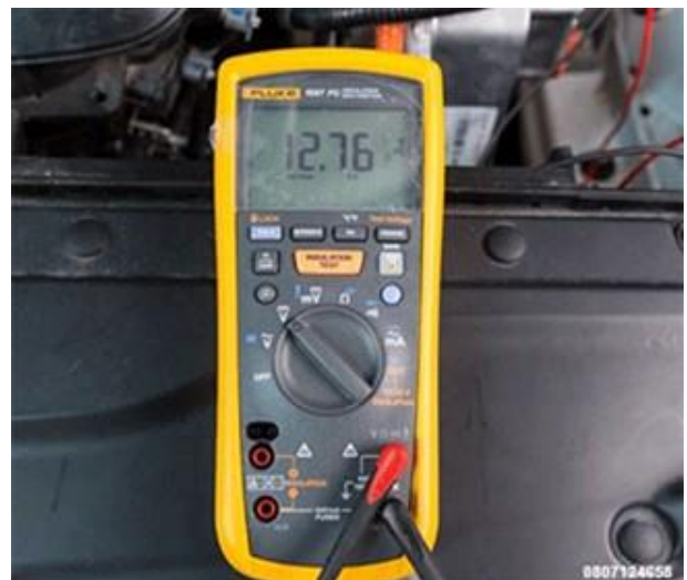
Figure 10 – PHEV Circuit Testing
