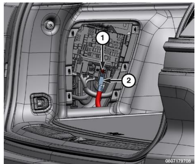
Figure 18 – 12-Volt Cable at Rear PDC
