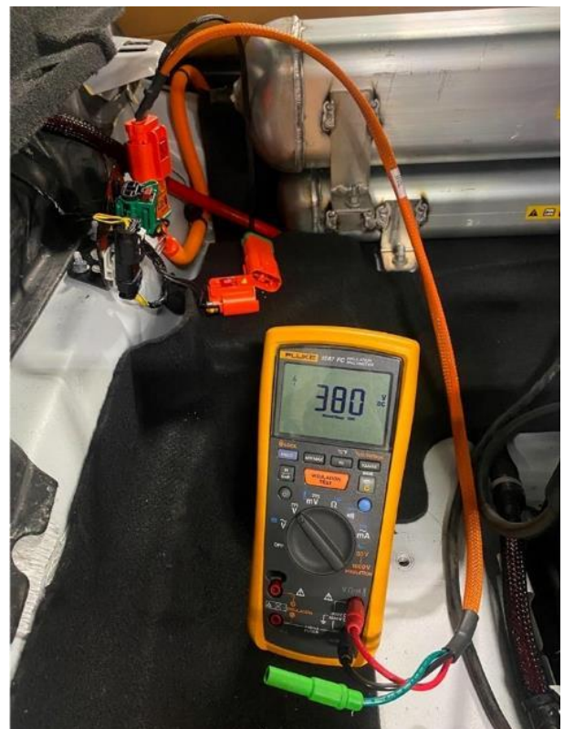
Figure 12 – PHEV Circuit Testing
