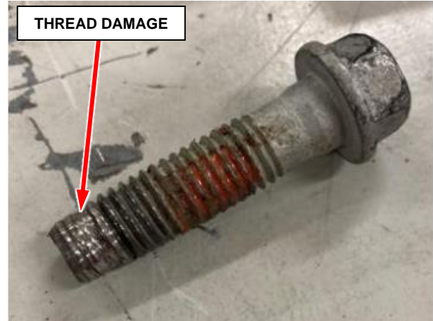
Figure 21 – Inspect Bolt Threads
