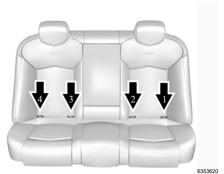
1. Locate the rear seat child seat anchors as shown above.
