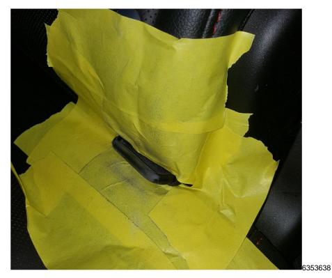
3. Mask off the area surrounding the anchor using painter's tape, paper, cardboard, or whatever you find convenient and appropriate, as long as it ensures the seats will not be damaged or painted during the repair. Example shown above with painter's tape.
