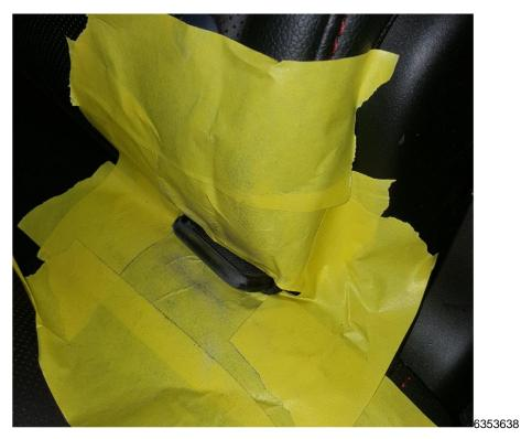
3. Mask off the area surrounding the anchor using painter's tape, paper, cardboard, or whatever you find convenient and appropriate, as long as it ensures the seats will not be damaged or painted during the repair. Example shown above with painter's tape.
