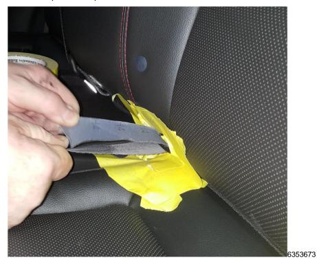
4. Using a strip of emory cloth or sandpaper 1 inch (25mm) or less in width, sand the powder coated surface down to bare metal. It is only necessary to sand down the part of the anchor that is parallel to the seats – no need to do the parts of the anchor that go through the seat cushion.
