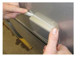
Use the plastic windshield tool to pry the cover off the sidewall.
