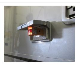
Plug into 120V shore power, allow for up to 60 seconds for surge protector delay, then polarity test the outlet.
