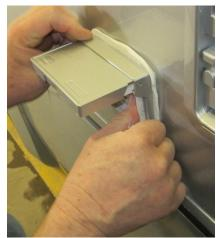
Press cover firmly in place and resecure with original screws.
