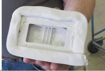
Place a single layer of butyl tape (129-0159) around the perimeter of the cover.
