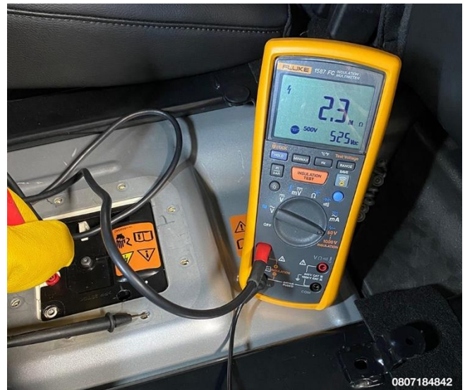
Figure 11 – Measure and Record Isolation Resistance Between HV Positive Test Point and Chassis Ground
