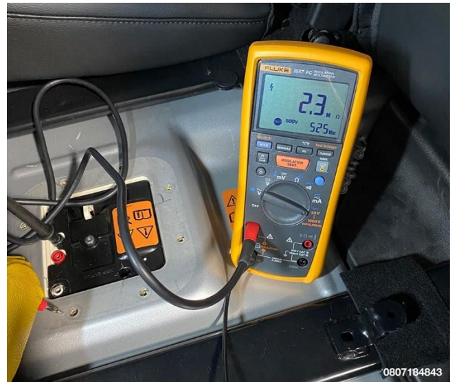
Figure 12 – Measure and Record Isolation Resistance Between HV Negative Test Point and Chassis Ground
