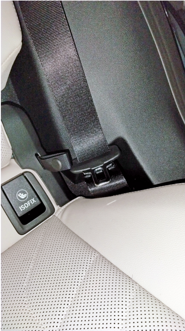
The safety belt webbing is slightly clamped by/pinched under the C-pillar trim at the bottom. The latch is held in a low position. NOT OK
