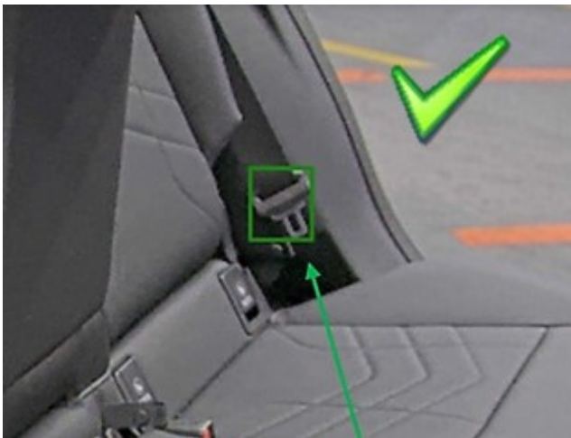
Safety belt installed correctly. OK
