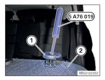
• Continue to hold the lock shown above unlocked with the special tool and at the same time guide out the guide sleeve (1) from the seat (2).
