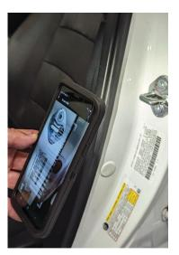
Align the VIN barcode in the door jamb to the outline displayed on the screen.
