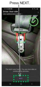
A green check mark will be displayed in the top right of the screen when the application is able to verify the repair.
