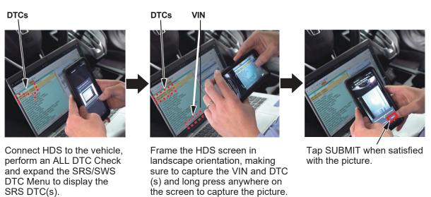
8. After the picture of the HDS screen is submitted, the application displays front seat belt buckle DTCs specific to the buckle being worked on. Review the DTCs retrieved from the vehicle to determine if the DTCs match any of the DTCs displayed in the list on the application screen.
