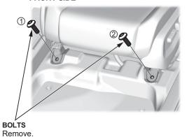
8. Lift and move the seat back while leaning the seatback into the rear door opening to lay the seat on its side.
