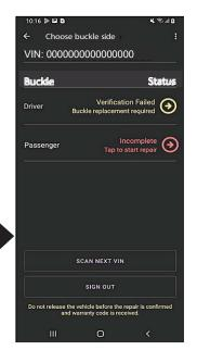
The status for the buckle will display "Verification Failed Buckle replacement required" in yellow. When a buckle becomes available, repeat steps 1-4 of the inspection procedure to get to the Status Screen. Select the yellow arrow to the right of the status to resume the Seat Belt Buckle Replacement Procedure.
