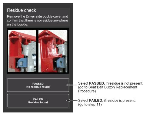
11. When **FAILED** is selected, the application will request a picture of the residue.
