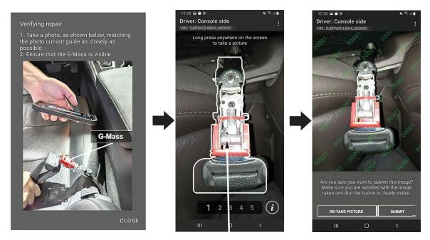
With the buckle still latched, pull down on the buckle and frame the picture using the application's cut-out guide.
