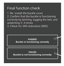
Select PASSED, if the buckle is functioning correctly and no SRS indicators or buckle DTCs have been introduced. (Go to step 7)
