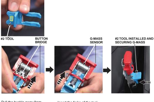
Pull the buckle away from the center console to prevent scratching/damaging the console when installing the #2 tool.
