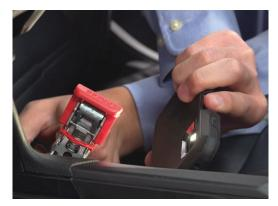
NOTE: Examples of buckles with residue that would cause the buckles to fail the residue check.
