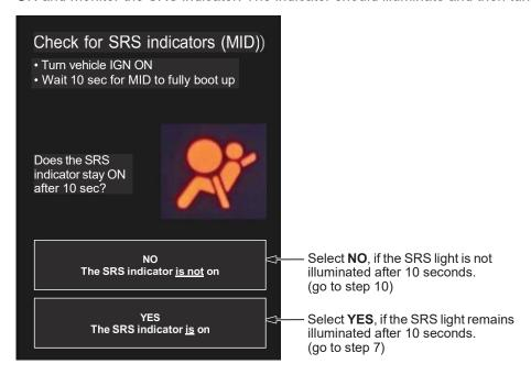
7. When **YES** is selected in the previous step, the application will request a picture of an ALL DTC CHECK from the HDS screen.
