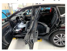
9. With the seat laying on its side, remove the seat belt buckle from the seat frame.
