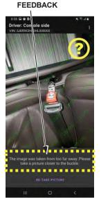
If the application is unable to verify the repair, a "?" or "X" will be displayed in the top right corner of the screen and feedback will be provided on the bottom of the screen to assist in improving the next picture retake.
