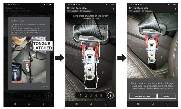
Insert the Seatbelt Tongue into the buckle and confirm it is latched. Pull up on the seatbelt to provide a clear view of the buckle. Frame the picture using the app's cut-out guide. Long press on the screen to capture the picture.
