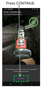
A green check mark will be displayed in the top right of the screen when the application is able to verify the repair.
