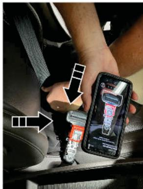
Move the camera away from the seat bolster, making sure the camera is parallel with buckle and both blue tabs are visible in the picture.
