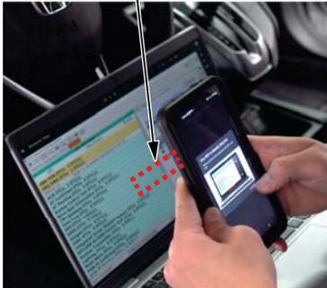
Connect HDS to the vehicle, perform an ALL DTC Check and expand the SRS/SWS DTC Menu to display the SRS DTC(s).
