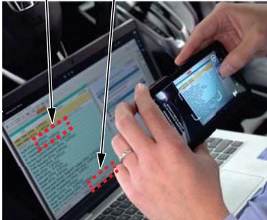
Frame the HDS screen in landscape orientation, making sure to capture the VIN and DTC (s) and long press anywhere on the screen to capture the picture.
