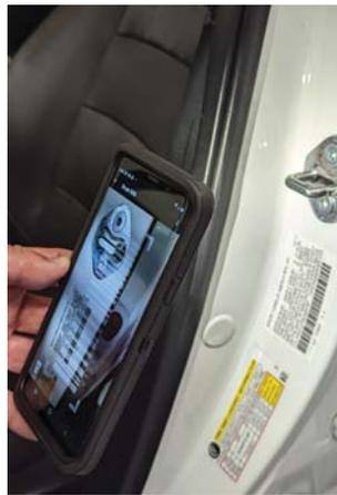
Align the VIN barcode in the door jamb to the outline displayed on the screen.
