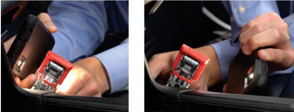
NOTE: Examples of buckles with residue that would cause the buckles to fail the residue check.
