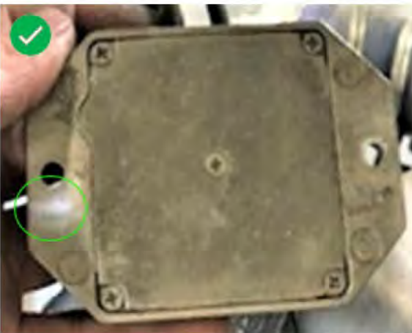
SENSOR COVER DIRTY AND ROUGH BUT SMALL WHITE SPOT NOT TOUCHING THE EDGE - CLEAN & REINSTALL
