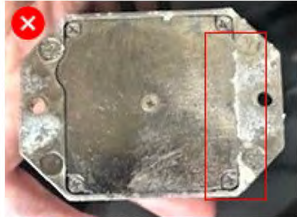
WHITE CORROSION AT ONE EDGE - REPLACE
