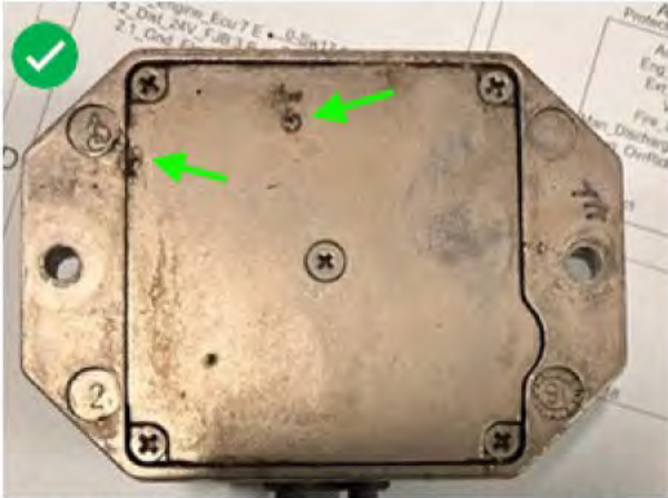
SUPERFICIAL BLACK SPOTS ARE OK - CLEAN & REINSTALL
