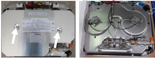
7. Visually inspect the gas tubes connecting the gas valve to the burner orifice holder for any cracks, splits, etc. Ensure no gas lines are loose by <u>gently</u> pulling the tubing along its axis away from each brass nut. <u>Use only two fingers.</u> If any gas lines are loose, stop the recall kit process and request a replacement unit by contacting Suburban Tech Support at 574-247-9235, option 5.
