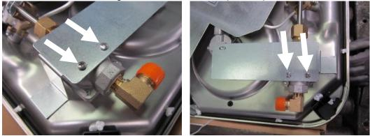
12. Apply force of 15 lbs. minimum to regulator bracket to firmly adhere VHB tape. (Minimum application temperature of 50°F. If necessary, heat tape and application surfaces prior to adhesion.)
