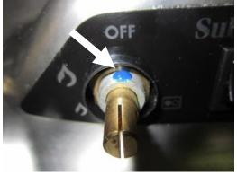
20. Install top nut and torque to 20 in-lb.
