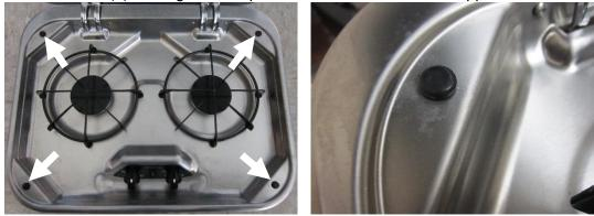
3. Using a #2 Phillips screwdriver, loosen the screws under each bumper. This will retract the clamping mechanism that attaches the cooktop to the countertop.
