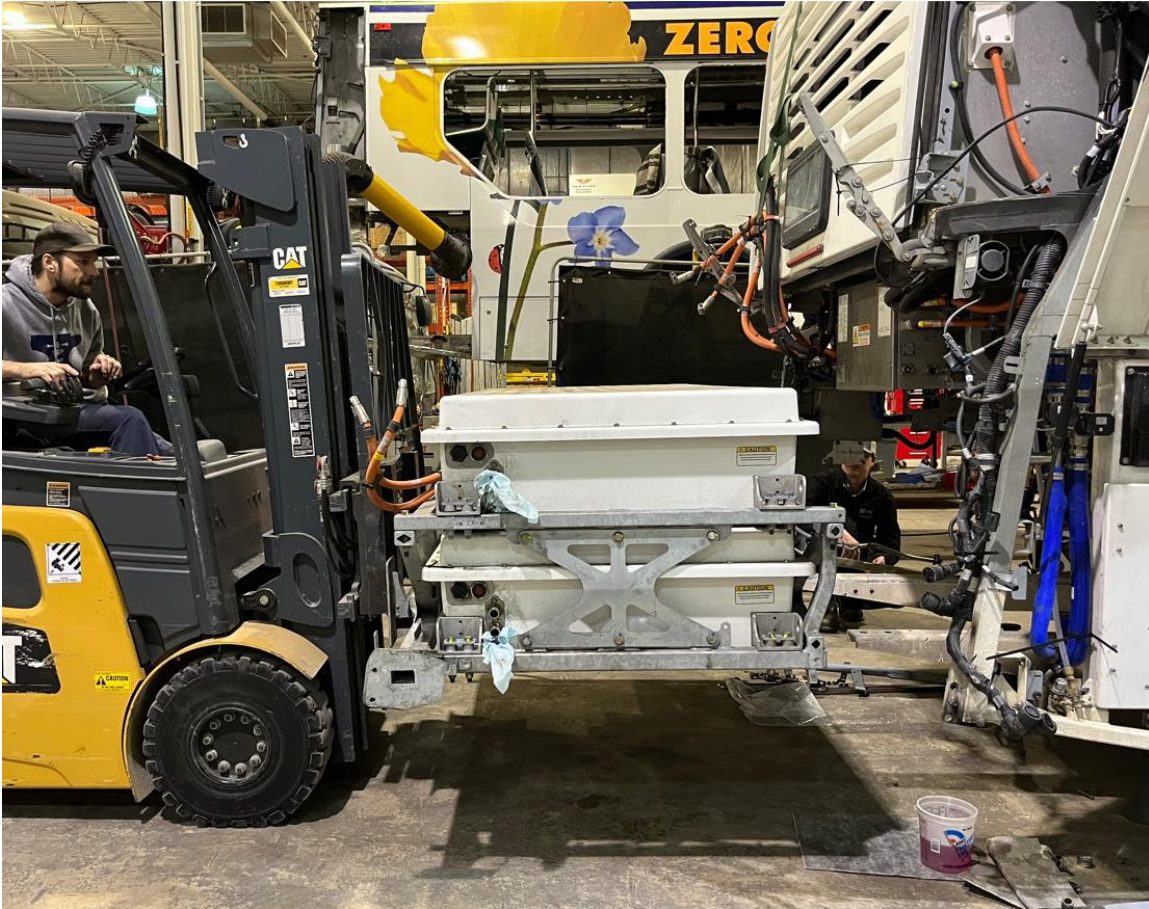
Figure 10: Installing ESS Enclosures
