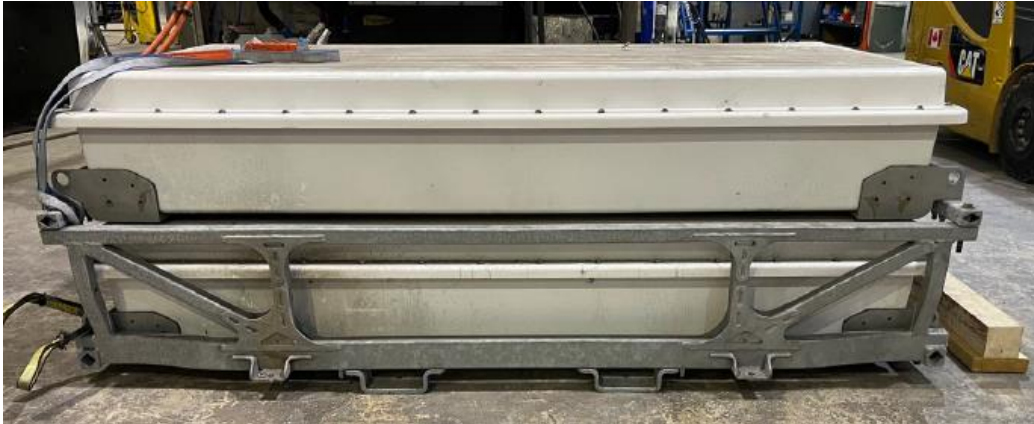
Figure 13: ESS Enclosures to be Reworked
