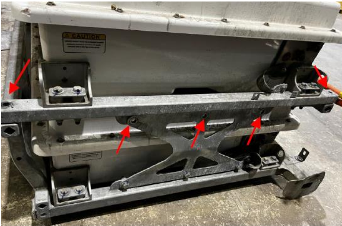
Figure 14: Remove Upper Cross-Brace Hardware (5 Places Each Side)
