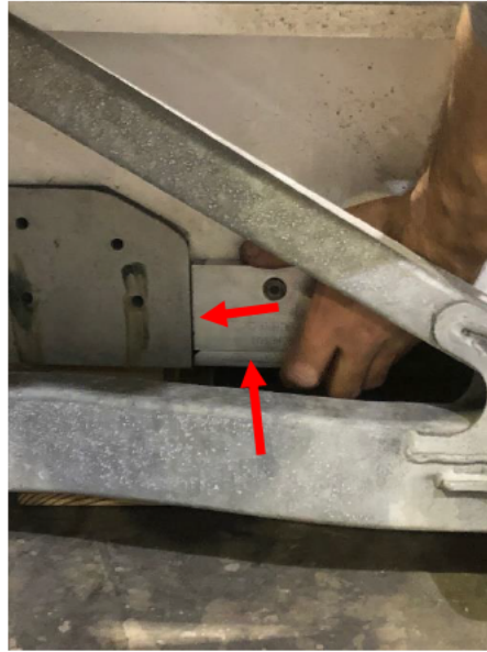
Figure 21: Place Fixture Against Corner Bracket as Shown
