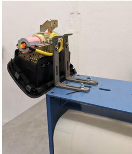
**STEP 1-** Peel the Sponge Tape and remove the harness clip from the retainer bracket by pushing the tangs inward with a flat-blade screwdriver as shown below. Always remove any Sponge Tape adhesive residue from the airbag mounting bracket using mild solvent on a clean shop cloth.
