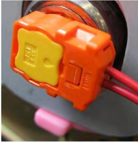
Once alignment is confirmed, push down firmly to engage the connector. When fully seated, press down on the yellow tab locking the connector to the inflator.
