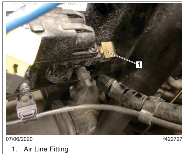
Fig. 9, Loosening the Brake Chamber Air Line Fitting
