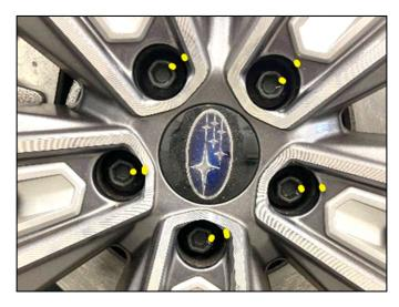
STEP 2: Using a Digital Torque Wrench, set the torque wrench to 90 ft-lbs (122 Nm). CAREFULLY torque ALL wheel bolts on ALL wheels in the pattern shown below.
