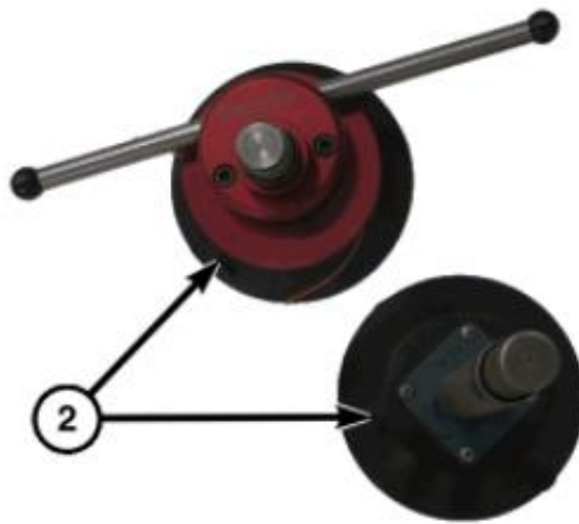
Figure 17 – Rotating Wire Windshield Removal Tool
