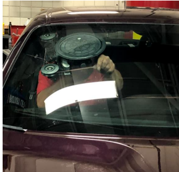
Figure 18 – Rotating Wire Removal System
