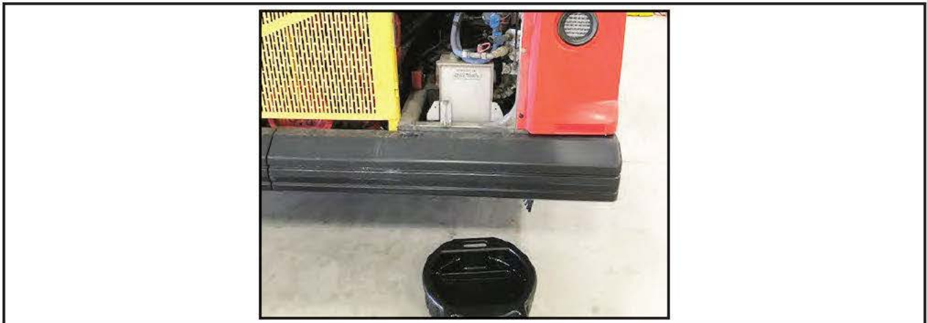
Figure 1 - Place Container to Collect Hydraulic Oil
