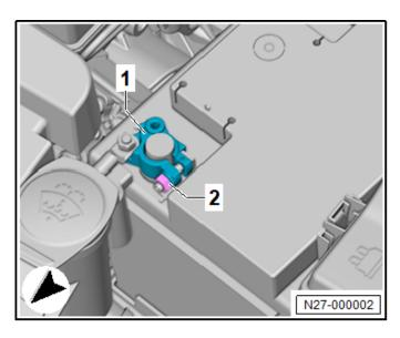
• Loosen the nut <2> several turns and remove the positive terminal battery clamp <1>.
