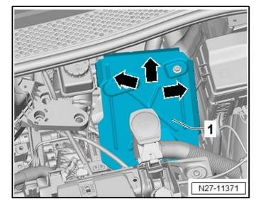
• Insert the battery into the battery tray <1> so that the battery clamping strip touches the rear and side stops <arrows>.
