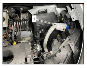
• The washer fluid filler neck will have to be unclipped and moved to the side.
