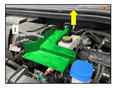
When removing the high-voltage connection cover <1> the cover has to lifted up <u>at the</u> <u>connection</u> to the firewall in the <direction of arrow>.
