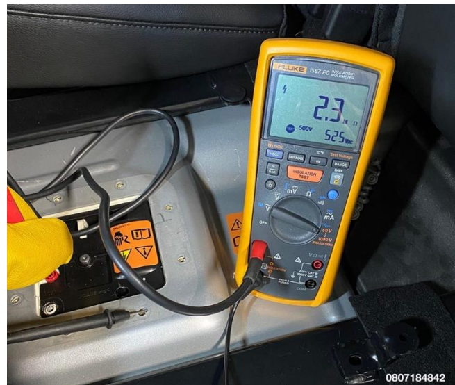
Figure 42 – Measure and Record Isolation Resistance Between HV Positive Test Point and Chassis Ground
