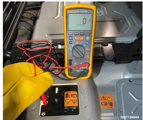
Figure 6 – Measuring at High Voltage Test Points
