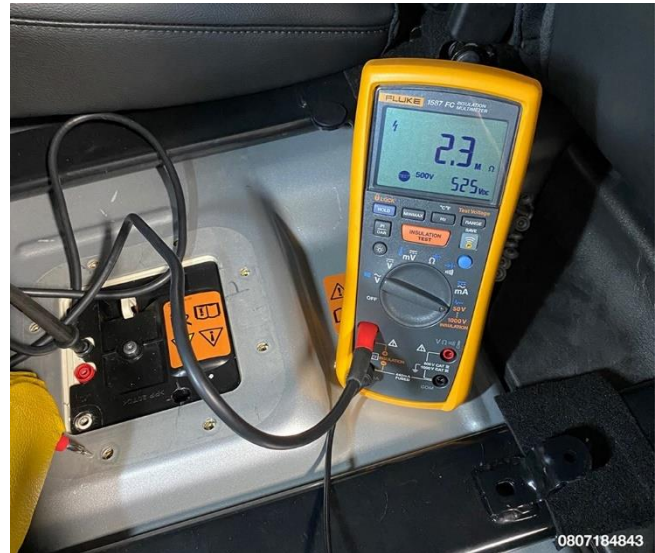
Figure 43 – Measure and Record Isolation Resistance Between HV Negative Test Point and Chassis Ground
