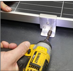
**6.** Repeat the process for the other brackets which completes the reworking process of the Type B mounting bracket.
