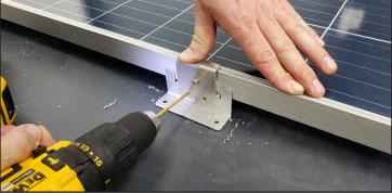
**6.** Drive the other two #12 screws into the recently-drilled holes and secure the add-on bracket to the pre-existing bracket.
