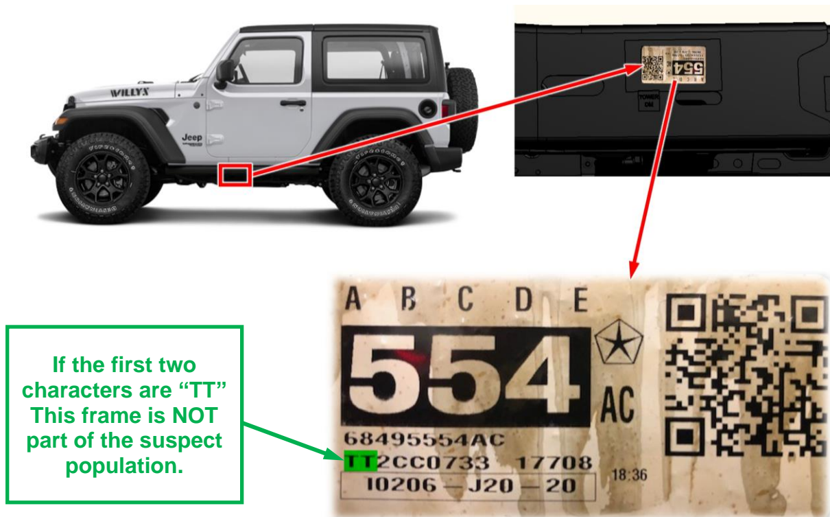
Figure 2 – Front Reinforcement Crossmember
