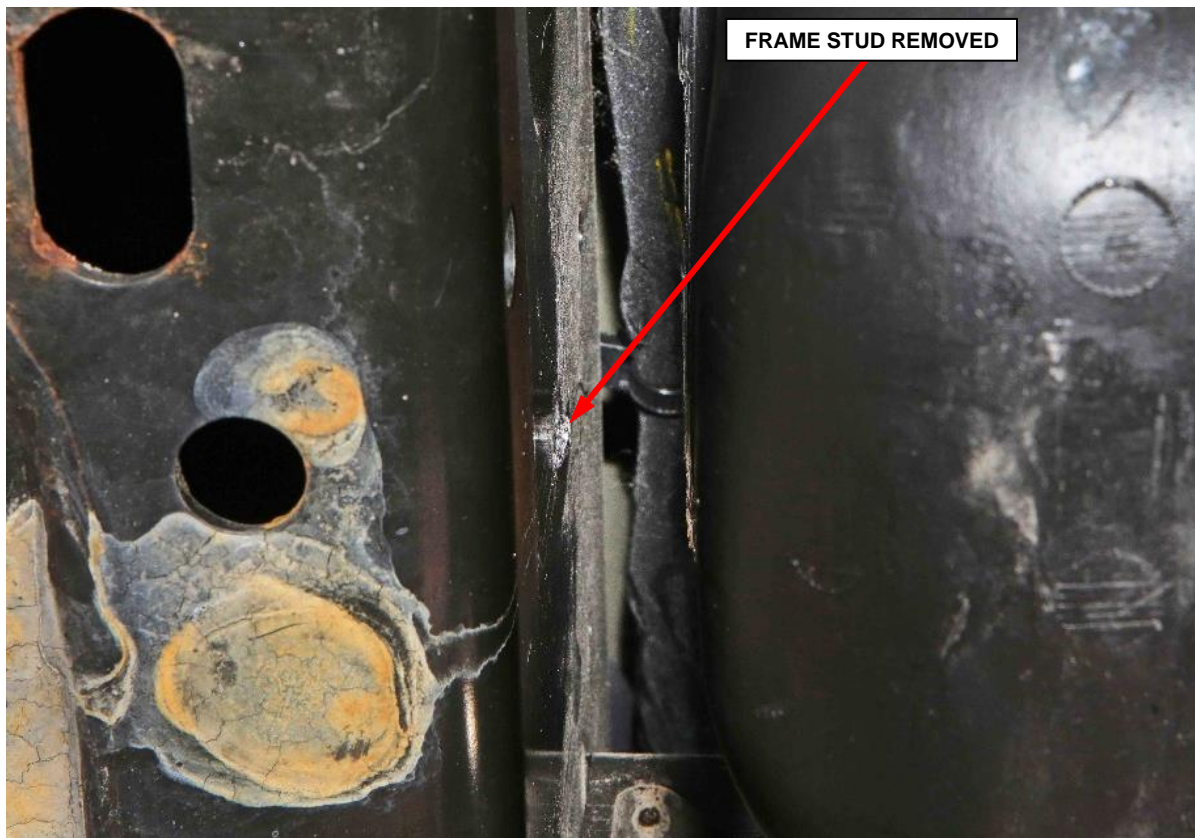
Figure 8 – Frame Stud Removed
