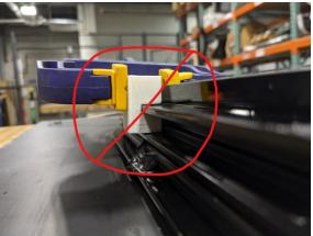
Figure 15b: Drill jig clamped incorrectly.
