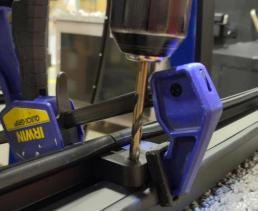
Figure 34: Drill aligned in drill jig.
