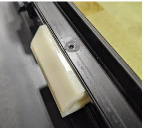
Figure 4a: Blade scraper removing sealant.
