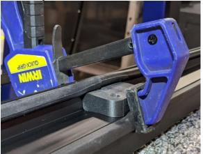
Figure 33a: Drill jig clamped in place.
