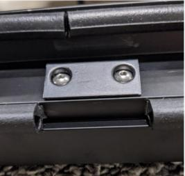
Figure 40a: Blade scraper cutting seal.
