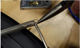
Figure 11a: Hold the ER bar and pull the spring hook with the pliers.
