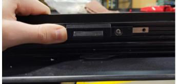
Figure 20: ER bar held in place with enough room to install ER handle cable.
