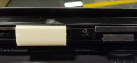
Figure 24: Offset locator block with gap between ER latch and block.
