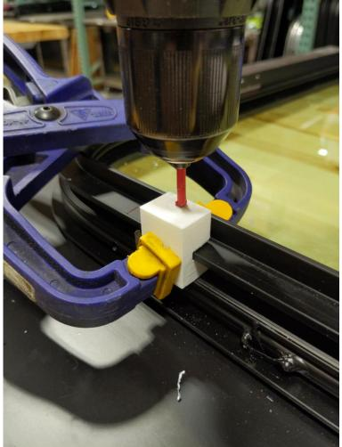
Figure 17: Additional split pin hole drilled to proper depth.
