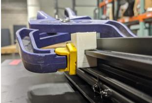
Figure 15a: Drill jig clamped correctly.
