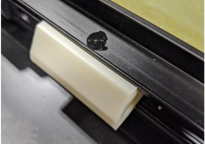
Figure 27: Sealant applied to split pin. 17. See Figure 28 for the complete updated ER bar in the mainframe assembly.
