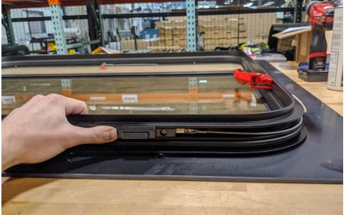
Figure 9: ER bar slid towards ER handle creating slack in ER cable.
