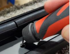
Figure 35: Deburr holes after drilling.
