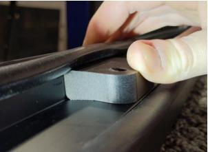
Figure 31b: Drill jig sitting on subframe sill.
