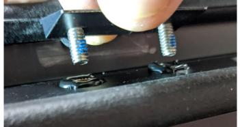
Figure 39: Install screws into rivet nuts.
