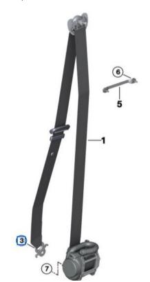
If the seat has been removed from the vehicle the safety belt mounting screw must be replaced (9909471 screw).
