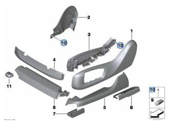
Seat plastic covers are held by blind rivets which may have to be replaced for access (7042164 blind rivet).
