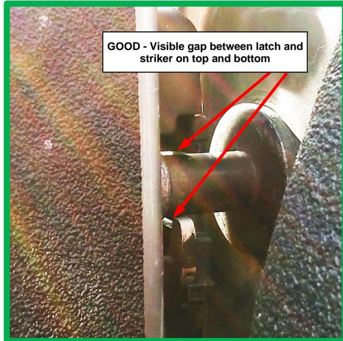
**Figure 1 – Striker with Proper Clearance**
