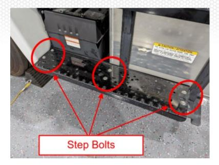
**16.** Reinstall the lower cab step and all six fasteners removed in step **1.** Tighten the fasteners to the specified torque.
