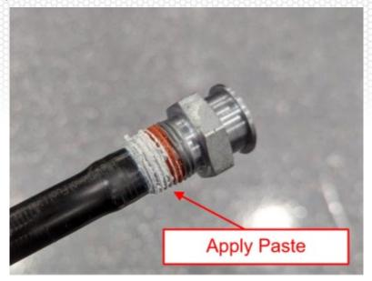
**10.** Install the fuel pick up tube in the fuel tank and tighten to the specified torque.
