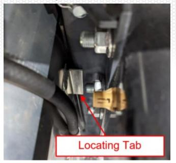
**12.** Reposition the two fuel tank straps and install a new SZ177-12005 nut on each strap. Do not tighten the nuts at this time.
