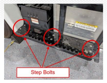
**2.** Remove the ten bolts attaching the upper cab step and remove the step. Retain the 10 bolts and upper step for reassembly.
