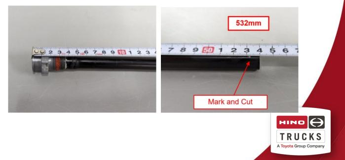
**9.** Apply a thin coating of TFE paste to the threads of the fuel pick up tube fitting. Use care as to not allow excess paste under the threaded portion as this can contaminate the fuel tank.
