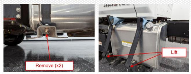
**6.** Slide the fuel tank rearward on the chassis until the fuel pick up tube on the rear of the tank clears the rear edge of the cab.
