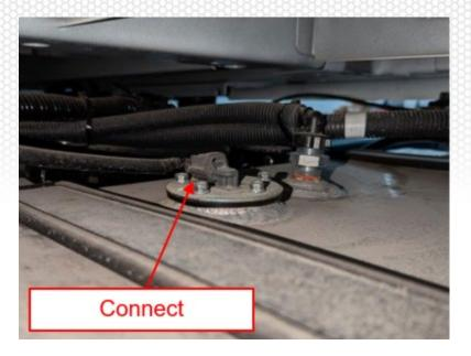
**14.** Reconnect the fuel pick up line by pushing the line back into the pick up tube on the fuel tank. Slide the locking ring removed in step **4** around the connection and ensure it is fully seated.
