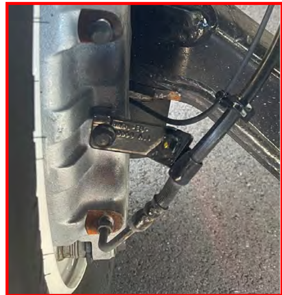
Figure 5 - Caliper-to-hose bracket (Correct)
