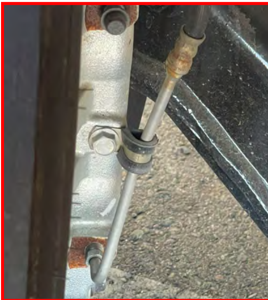
Figure 4 - Caliper-to-hose clamp (Incorrect)
