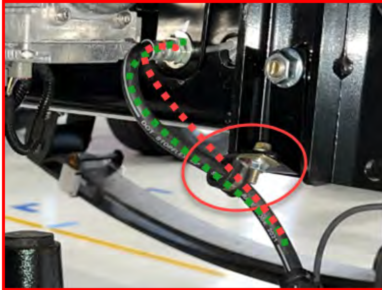
Figure 15 - P-Clamp Securing the Rubber Brake Line Gradual Bend (Green) vs Sharp Bend (Red)
