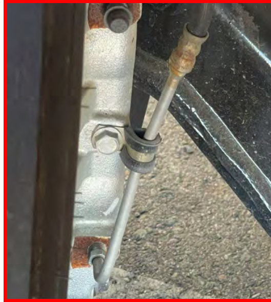
Figure 4 - Incorrect Caliper P-Clamp
