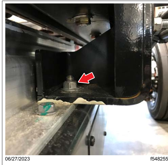
Fig. 7, Battery Pack Mounting Fastener Location
