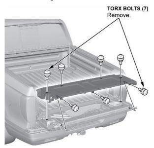
• Using a TORX T40 bit, remove the bolts, and then remove the tailgate trim.
