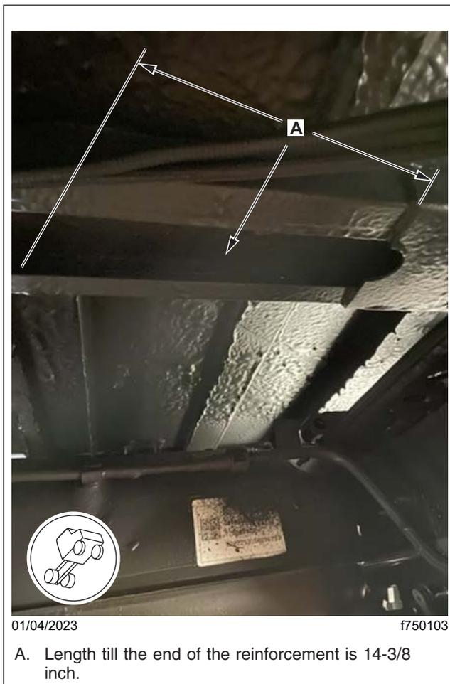
**Fig. 3, Installing the Joist Reinforcement**
