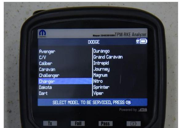
**Figure 6 – Vehicle Model Selection**
