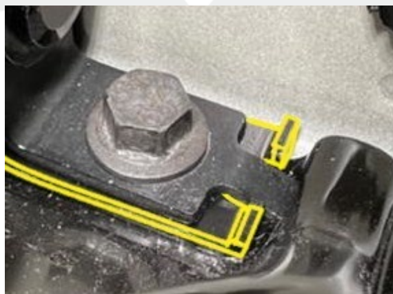
✓ Figure 5 — Guide pin aligned with slot
