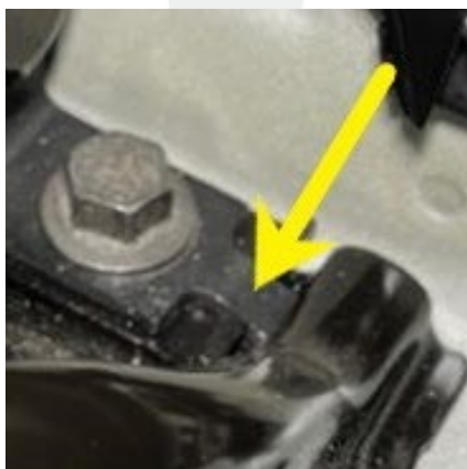
✓ Figure 6 — Guide pin in hole of penthouse rail
