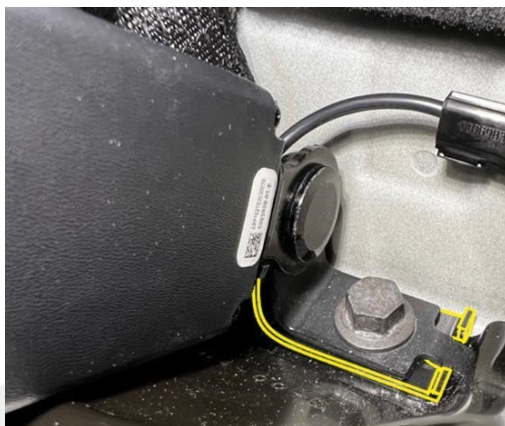
✓ Figure 4 — Anchor has belt to RH side
