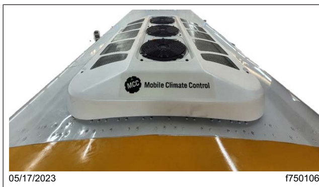
Fig. 4, Vehicle Equipped with Factory-Installed Roof-Top A/C Unit
