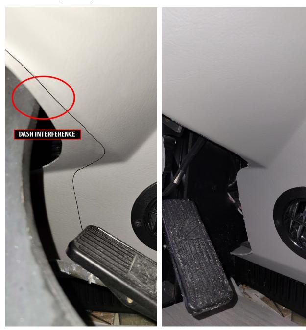
2. Using an air saw or a similar cutting device, cut slowly along the marks made in the previous step, making sure no wires are in the path of the blade. If you try to cut too fast, you may melt the plastic back together.
