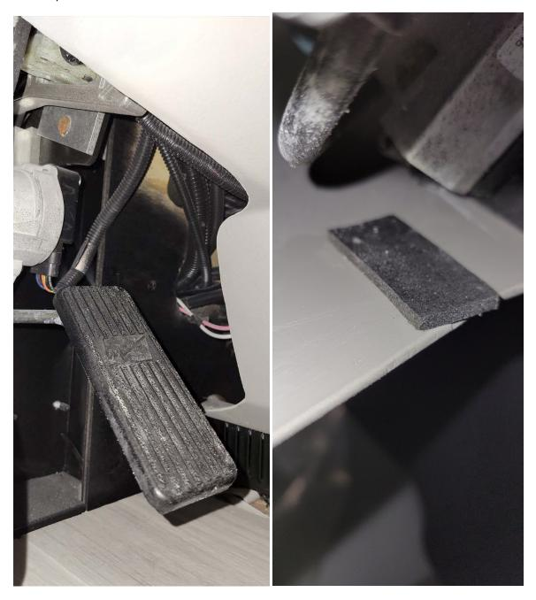
4. Add a piece of foam tape to the back side of the dash in line with the brake pedal arm. This will eliminate dash rattling if the pedal arm is still close while driving with the pedal assembly fully extended.
