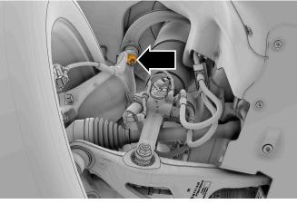
• **CAUTION:** When using a torque wrench with an offset socket, rotate the offset socket to exactly 90° from the body of the torque wrench. Other angles will cause an inaccurate torque measurement.
