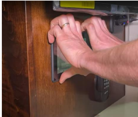
Place fingers on top edge of Touch Screen and apply pressure down and out
