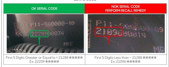
NOTE: Suspect Subframes must be Revision -09 AND the First 5 Digits of the Serial Code less than 21288.
