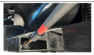
NOTE: A 12" Extension is required for proper drill angle and clearance.
