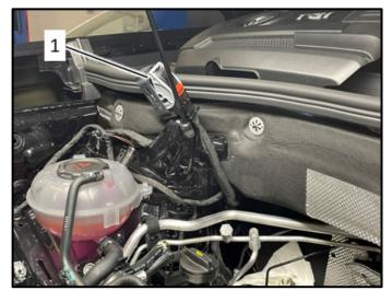
Secure the ABS control module connector <1> out of the way.
