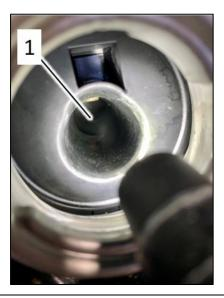
Fuel condensation formed on adapter cap <1>.
